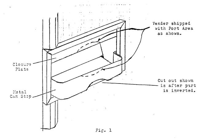
1. Vender is shipped with "cut outs" (dotted lines) as shown on Closure Plate and Can Stop.
